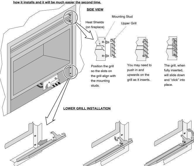
Hold the grill at an angle and insert the lower slot over the bushing on the fireplace (both sides). You may need to press on the grill to get the tab over the bushing (this prevents the grill from accidentally falling off).
